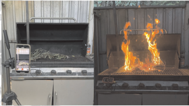
Left: Flammability testing apparatus. Beefeater 1100 between two windbreaks with a sample preparing for burn. iPhone 14 on tripod to record flame heights. Right: Active burning post blowtorch on distal end for 10 secs.
